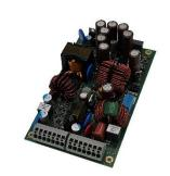
The brand new HFBC250-2DW with 250 W power offers an ultra-wide input range from 14.4 V to 154 V and is ideally suited for power-hungry applications.
